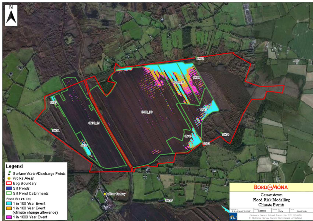
Figure 3.3-9 Carranstown Bog Pluvial Flooding, Rainfall Events
