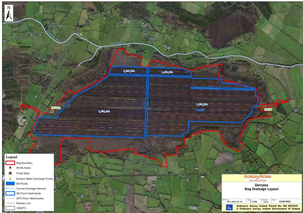
Figure 5.8.2 Derrylea Bog Drainage Layout
