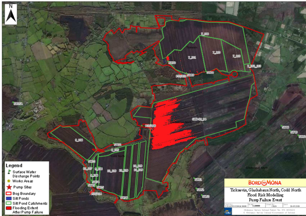
Figure 5.9.10 Ticknevin/Glashabaun North/Codd North Pluvial Flooding, Pump Failure
