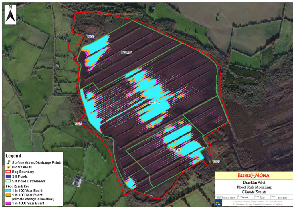
Figure 3.2-9 Bracklin Bog Pluvial Flooding, Rainfall Events
