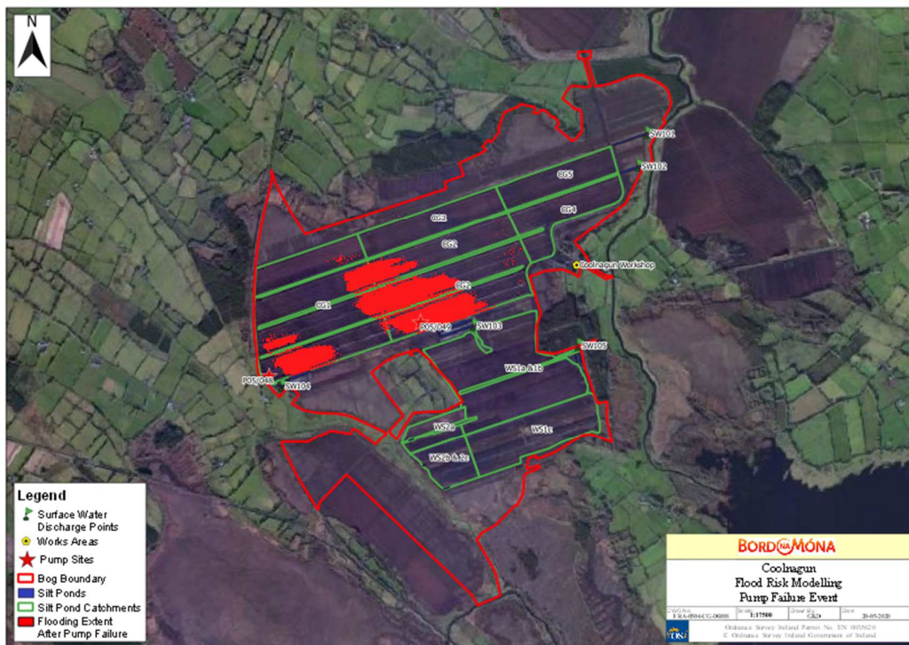
Figure 6.2.10 Cuil na Gun Bog Pluvial Flooding, Pump Failure
