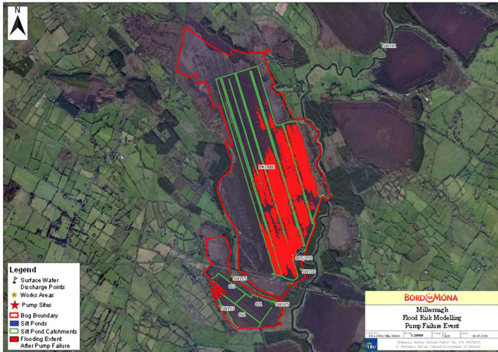
Figure 6.3.10 Milkernagh Bog Pluvial Flooding, Pump Failure
